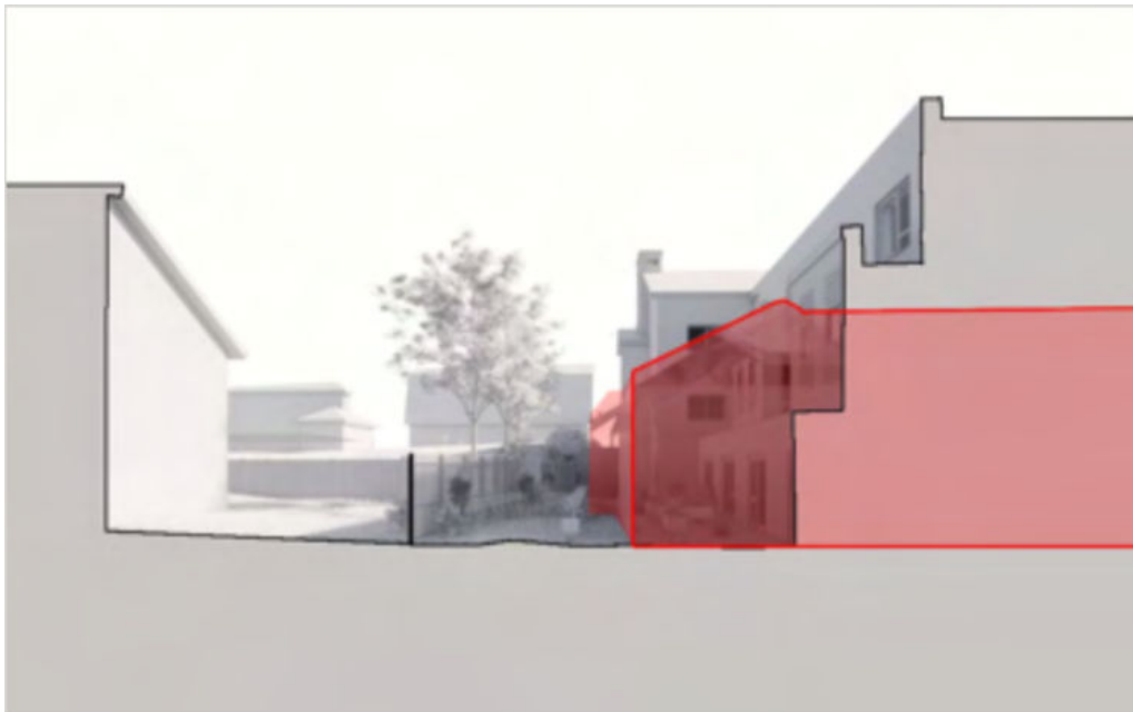
Comparative 3D Section view showing the existing building and proposed extension at the boundary shared with property No 6 Littlebrook.
